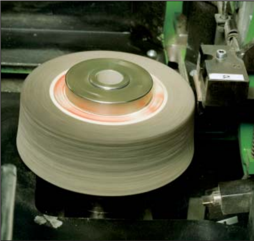
Fig 2 Machining the radius on a diamond segment
