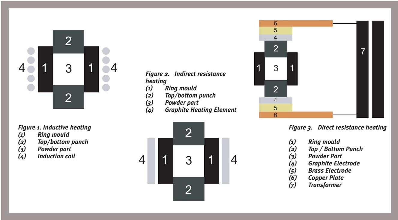
Up to now, this technology has been used mainly in the metal powder field with typical maximum temperatures of 1400°C.
